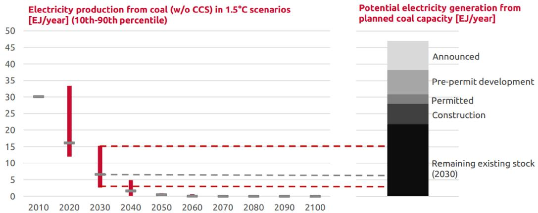
Note: Coal-fired power generation (without CCS) in a selection of 1.5°C scenarios. The ranges indicate the 10th to 90th percentile, while the grey line indicates median values. The median values show a rapid decrease of coal-fired power generation
